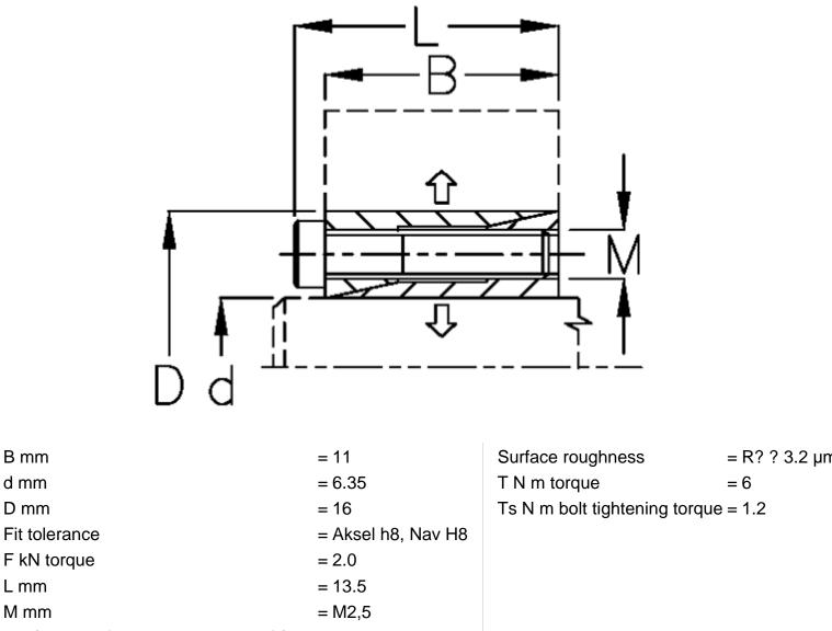
P N/mm2 surface pressure on shaft/hub = 55
